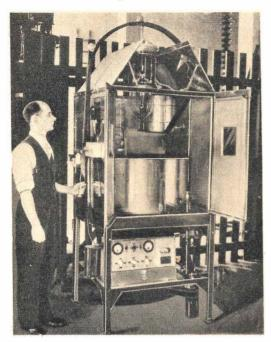
Designed for testing various materials, this "weatherometer" device can duplicate any weather condition such as rain, fog, desert heat, etc., by the mere turning of control knobs.
