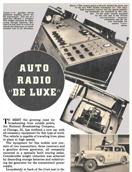
control panel and console, which houses the ultra-high frequency receiver and the specially designed four-stage high gain audio amplifier. To the rear, in the space usually occupied by the back seat, is a large compartment containing a fifty-watt transmitter, used for stationary broadcasts. A forty-watt
