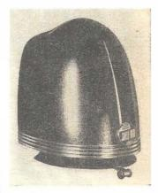
Entirely independent of the motor cooling system, the automobile heater shown above burns gasoline in a patented sealed metal chamber. The fuel is drawn in through a line tapped tuel is drawn in through a line tapped to the carburetor of the auto and, when mixed with air in a special venturi, burns as an extremely hot gas. The gas is ignited by turning on an electric heating element, which automatically shuts off in about 90 seconds.
