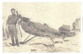
Mounted on spring-set runners to insure easy riding over rough ice and powered by an old motorcycle engine, this air-sled carries builder Lloyd Knoepke one mile in 43 seconds.
