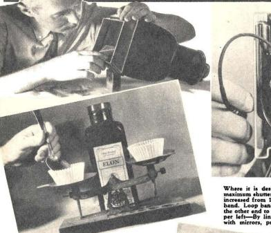
Where it is desired to stop motion, the normal maximum shutter speed of any good camera can be increased from  $1\frac{1}{2}$  to 2 times by use of a rubber band. Loop band over the setting lever and attach the other end to wire finder in manner shown. Uper left—By lining inside of enlarger lamphouse with mirrors, printing time can be reduced  $\frac{1}{2}$ 4.
