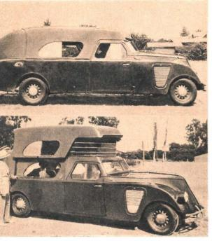
The roof of this streamlined auto (top) features a cleverly concealed magazine bed that furnishes the "bedroom" created when the roof is raised, as shown in lower photograph.
