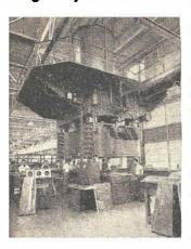
Featuring a pressure capacity of 5,000 tons, the world's largest self-contained hydraulic press (above) has been installed at the Douglas Aircraft plant in Santa Monica, Calif. The gigantic press is said to accomplish several thousand production operations in the shap-ing and forming of special parts that are used in building Douglas planes.
