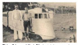
Walter Osborn and Hugh Fife devoted three years of spare time to building this 20-passenger streamlined "Silver Streak" train. Powered by a gasoline motor, the train travels 25 m.p.h.
