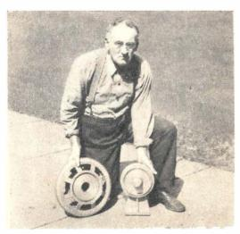
Daniel Slick exhibits the new auto wheel and snxle he invented to facilitate tire changing. Wheel locks onto axle by means of four steel pins and can be removed in a few seconds.
