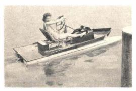
Using a 16-inch propeller, this pedal-operated boat can attain a speed of 10 m.p.h. A comfortable seat and ease of propulsion enables operator to make long trips without fatigue.
