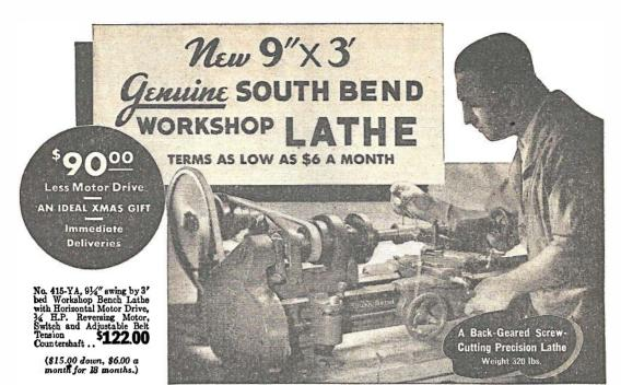
THE new 9-inch Workshop Precision Lathe is a back-geared, Screw Cutting Lathe, and has the same workmanship and materials as our larger, more expensive models,
