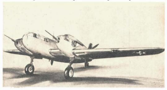
An artist's sketch of the XMF-1, a new type of pursuit plane developed for the U. S. Army Air Corps. Its twin pusher engines of 1,000 horsepower each are expected to drive it along at at over 300 m.p.h. Full armament consists of six machine guns.
