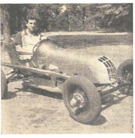
Powered by a motorcycle engine, this midget dirt track racer can travel 82 m.p.h. Builder Emanuel Forte is at the wheel.
